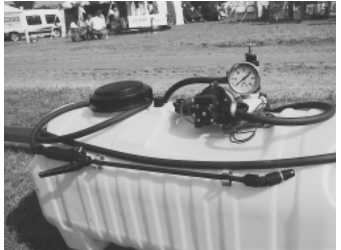
Sprayer tank, wand, pump and gauge.
