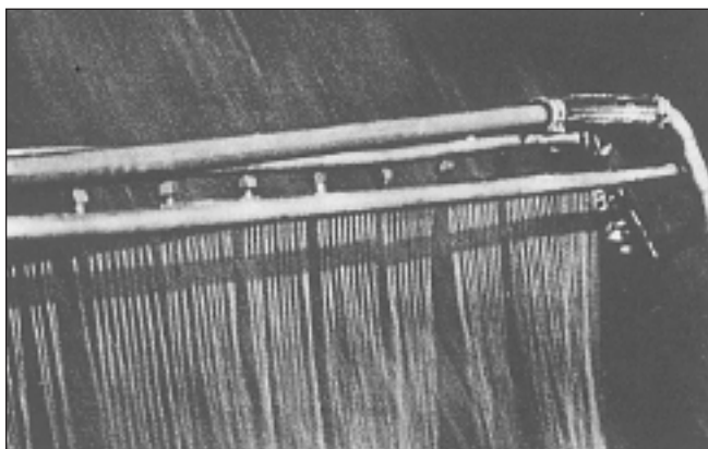
Figure 8-8. Microfoil booms are often used in aerial herbicide applications to reduce drift.
