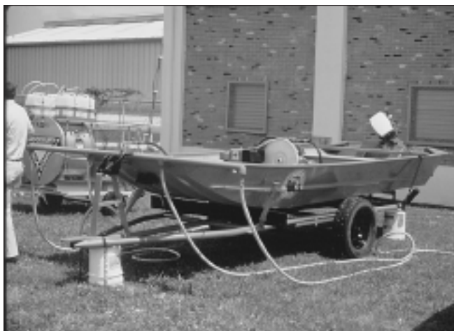
Figure 8-7. Deep water injection with long, weighted hoses can be used to overcome the effects of stratified water.
