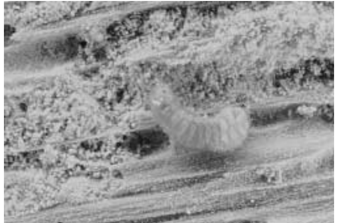
Figure 6.9. Anobiid beetle larva— E. peltatum . Note frass and damaged wood (USDA Forest Service).
